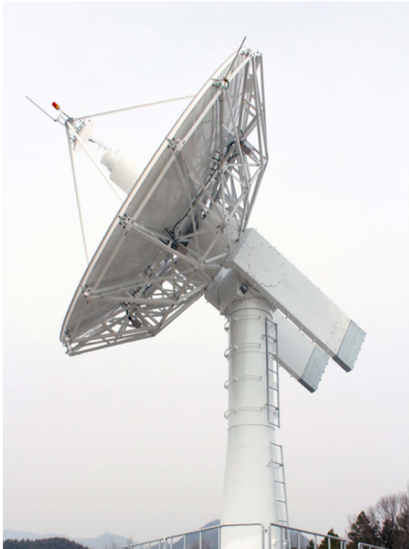
Figure 1. Satellite tracking antenna constructed at KASI for receipt of VAP space weather data.
